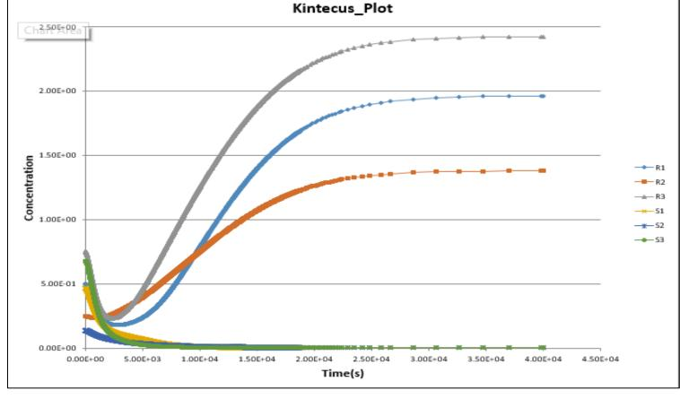
The graph to the left shows the different concentrations when R1=0.5 M, R2=0.25M, and R3 = 0.75M, while S1=0.47M, S2=0.14M, and S3=0.68M. As time passes, an excess of R
